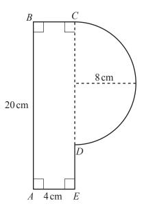
A uniform solid prism has cross-section *ABCDE* in the shape of a rectangle measuring 20 cm by 4 cm joined to a semicircle of radius 8 cm as shown in the diagram. The centre of mass of the solid lies in this cross-section.
