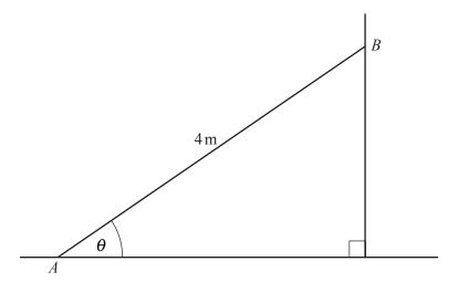
A uniform ladder AB of weight W N and length 4 m rests with its end A on rough horizontal ground and its end B against a smooth vertical wall. The ladder is inclined at an angle  $\theta$  to the horizontal where  $\tan \theta = \frac{1}{2}$  (see diagram). A small object S of weight 2W N is placed on the ladder at a point C, which is 1 m from A. The coefficient of friction between the ladder and the ground is  $\mu$  and the system is in limiting equilibrium.
